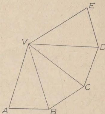
$$\text{Sup. lat. pir. reg. V. ABCDE} = \text{Sup. } \triangle VAB \times 4 = \frac{\overline{AB} \cdot a}{2} \times 4 = \frac{\overline{AB} \cdot 4}{2} \times a$$
