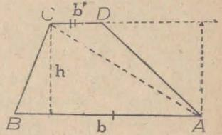
$$\begin{aligned} \text{Superficie del trapecio ABCD} &= \text{Sup. triáng. ABC} + \text{Sup. triáng. CDA} = \\ &= \frac{b \times h}{2} + \frac{b' \times h}{2} \end{aligned}$$
