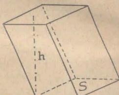
$$Volumen\ del\ paralelepípedo = Sup.\ base \times altura = S \times h$$
